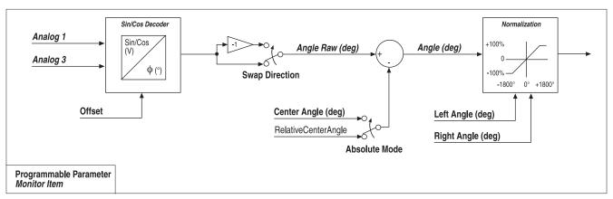
Fig. 6 Command Input Device "2" signal flow.
