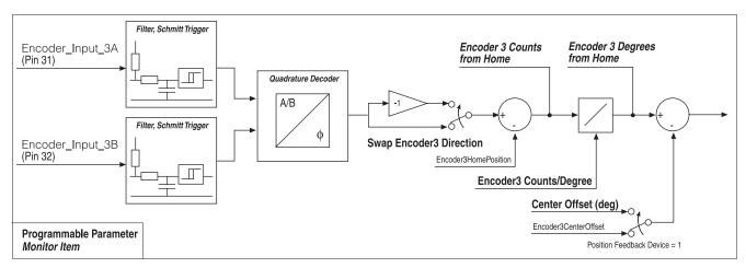
Fig. 11 Position Feedback Device "1" signal flow (Encoder 3 shown; Encoder 4 is similar).
