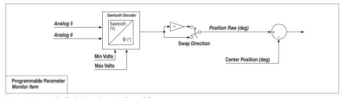
Fig. 13 Position Feedback Input Device "3" signal flow.
