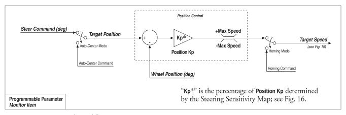
Fig. 14 Position Control signal flow.
