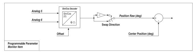
Fig. 12 Position Feedback Input Device "2" signal flow.
