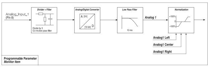
Fig. 4 Command Input Device "0" signal flow (Analog 1 shown; Analog 3 is similar).
