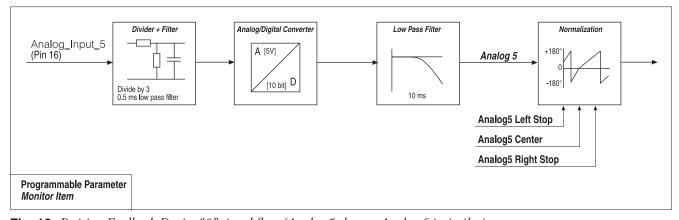
Fig. 10 Position Feedback Device "0" signal flow (Analog 5 shown; Analog 6 is similar).
