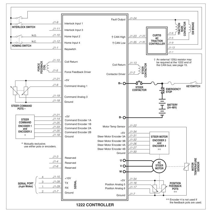
Fig. 3a Wiring diagram, Curtis 1222 electric steering controller.
