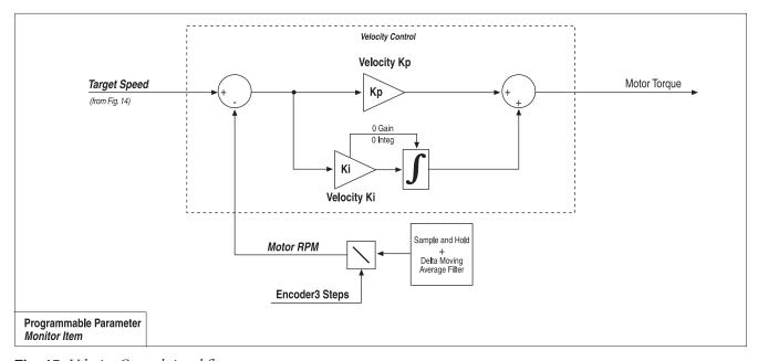
Fig. 15 Velocity Control signal flow.
