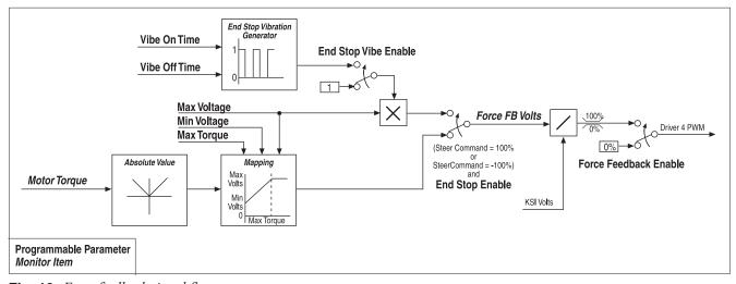
Fig. 10 Force feedback signal flow.
