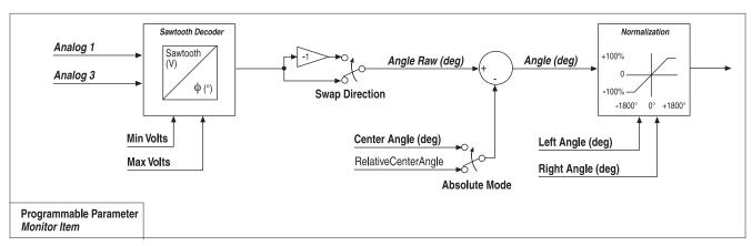
Fig. 7 Command Input Device "3" signal flow.
